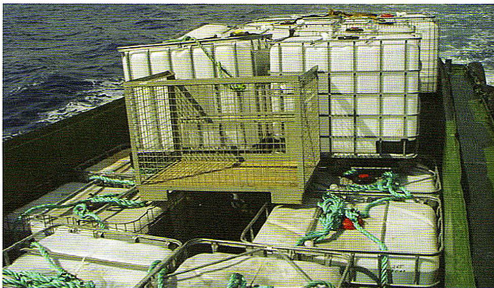
After spraying and cleaning tanks, the oil and water are collected in containers
